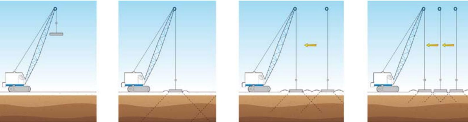
**Dynamic Compaction construction sequence**
