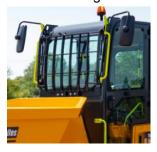
Wacker Neuson DW & DV Dumpers Skip Rear mounted guard
