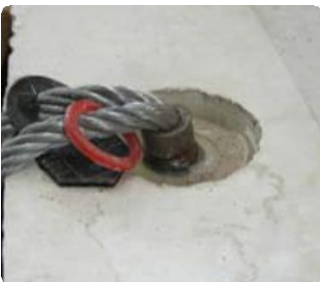
Wire slings bent over!
