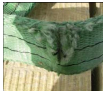
Sling damaged on sharp edges
