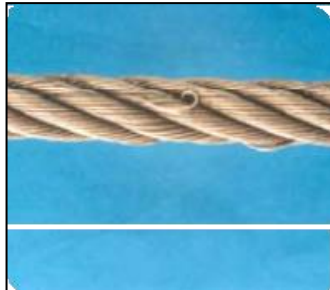
Damaged steel wire rope
