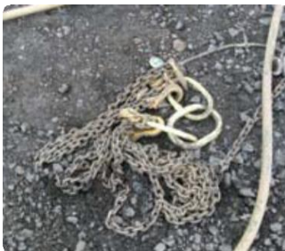
Badly stored chain slings
