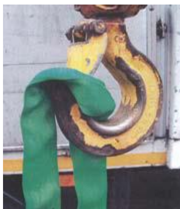
Conventional Safety Hook with Continuous Webbing Sling
