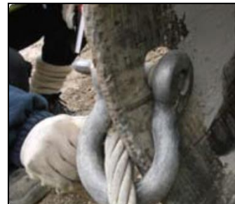
Shackle pin not flush with shackle – it must be 'finger tight'
